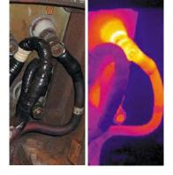
potential dangers associated with exposed high temperature surfaces in engine rooms.<sup>1</sup> The existing regulatory requirements have been highlighted to focus attention on companies' responsibility to ensure that the engine room systems are maintained in a safe condition and in compliance with relevant regulatory requirements at all times during operations.
