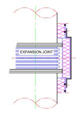
Figure A2-2 Insulation method on compensator part
