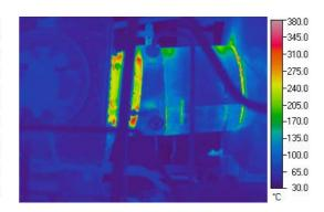
Figure 3. Exhaust gas outlet compensator to manifold(M/E)
