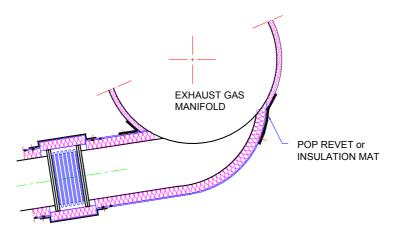
Figure A2-3 Insulation practice of discontinuous part
