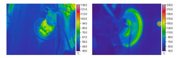
Figure 7. Boiler feed water valve close-up Figure 8. Boiler burning point
