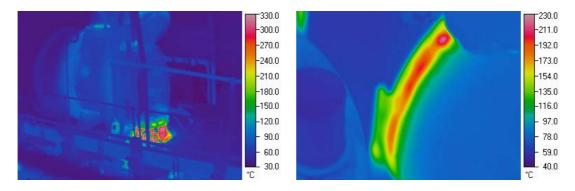
Figure 13 T/C inlet compensator Figure 14 M/E outlet compensator to manifold (missing part)
