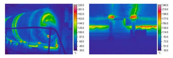
Figure 9 Exhaust gas manifold of M/E Figure 10 Exh. gas manifold support of M/E
