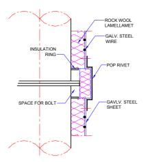
Figure A2-1 Insulation method on flanged part
