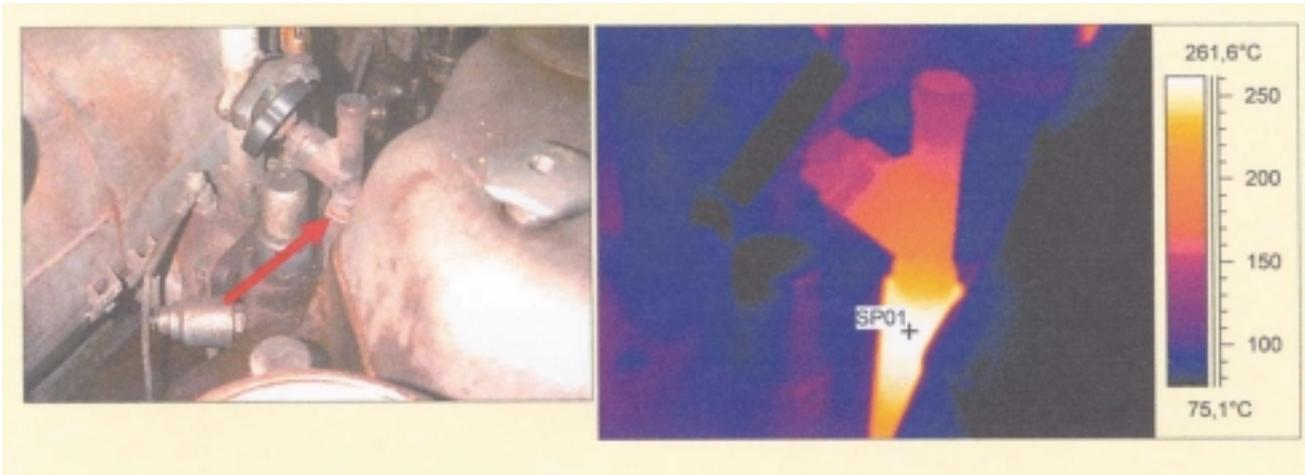
*Detail 1. Hot indicator valve. Area is only a few cm<sup>2</sup> and difficult to detect. It is advised to examine area around one chosen cylinder thoroughly, as many items will be identical on all other cylinders on that engine. Hot spot as indicated by arrow is 260°C.*
